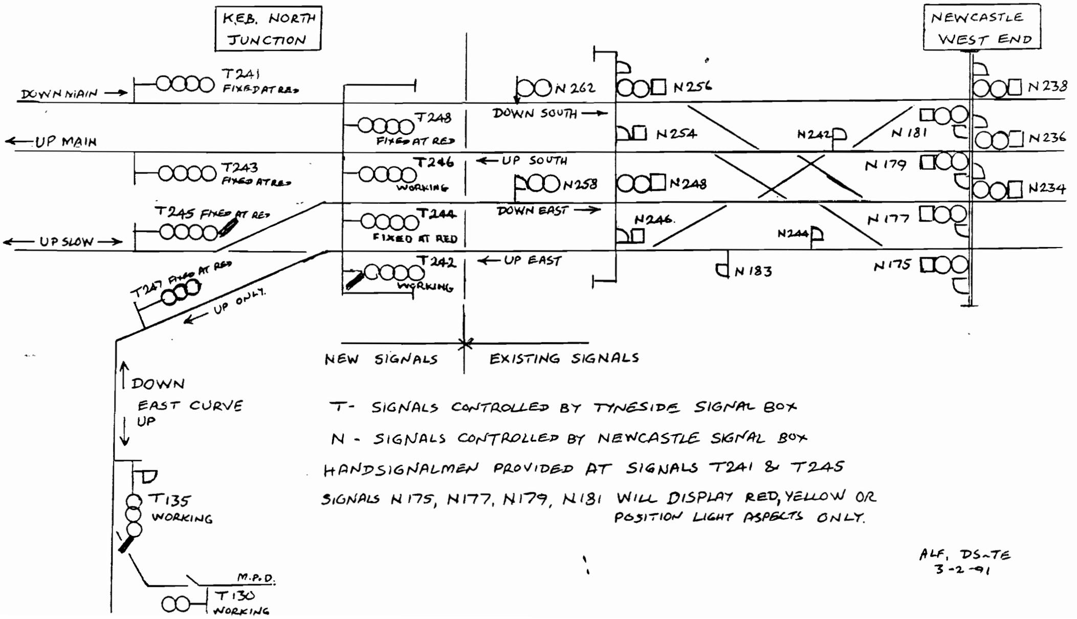
T - SIGNALS CONTROLLED BY TYNESIDE SIGNAL BOX
