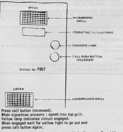
A vandal resistant telephone without handset has been installed adjacent to Ferryhill ground positionlight signal No.431 (Goods Yard to Down Passenger Loop). The action of opening the lid calls the (29)signalman.
